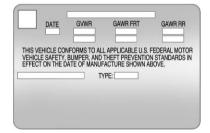
A vehicle specific Certification label is attached to the rear edge of the driver's door.
